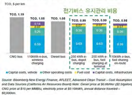
Figure 22: TCO comparison for the most likely e-bus configurations in a medium city
